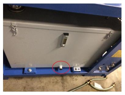
Or open the top cover of the oil reservoir, use an oil suction pump remove the old hydraulic oil. (notice don't drop the seal rubber inside the reservoir)
