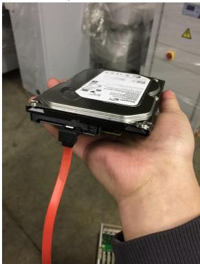
9. Connect cable 2, side B to same jack where the old hard drive connected to.
