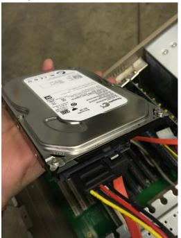
11. Connect cable 1, side B to the white connector where the small hard drive connected.
