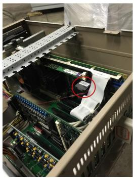
5. (REMEMBER WHERE THE HARD DRIVE WAS CONNECTED ON BOTH SIDE) Push on the little button on the hard drive and disconnect it from both side
