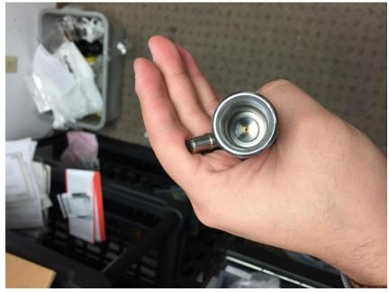
4. Slightly screw the cutting head and cutting body together until tight while keeping them put vertically so the orifice in it will not move. The new orifice will be ready to use now.
