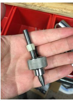
4. Put the end of the new nozzle into the cutting head then screw it back slightly until tight.
