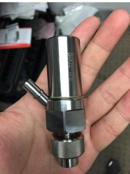
2. Take a new cutting head out from your spare package. Then screw it back to the cutting body.
